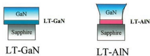
Figure 3. Macroscopic schematic structure of GaN grown on different LT buffer layers. In the case of LT-GaN, GaN is grown under constant tensile stress, while in the case of LT-AlN GaN is grown under compressive stress at the very initial stage, which then changes to tensile stress.
